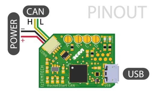
**Power**: between 4V and 17V. Protected against reverse polarity.
